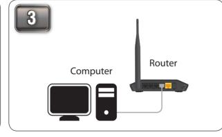
If you are currently using a router, disconnect all the cables connected to it before installing the DIR-605L. Unplug the Ethernet cable from your modem that is connected to your computer. Plug it into the LAN port labeled 1 on the back of your router. The router is now connected to your computer.
